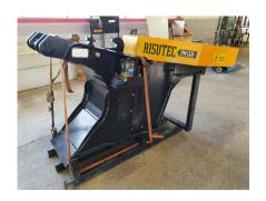
The device is easy to maintain, has centralized grease nipples and a hinged feeder. The machine is well protected against twigs and branches. The planting result is superior thanks to double-sided compaction.
